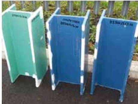
Interchar 2200 (shown as white areas) works well on flange edges to repair any damage
