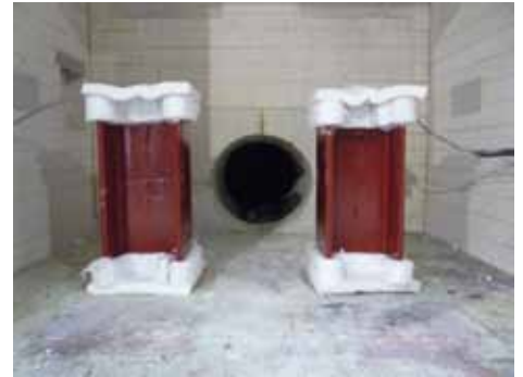
Test specimen after repair with Interchar 2200. Fire tested at International Paint's fire test facility
