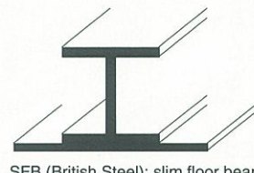
SFB (British Steel): slim floor beam
