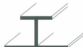
IFB (Arbed): integrated floor beam
