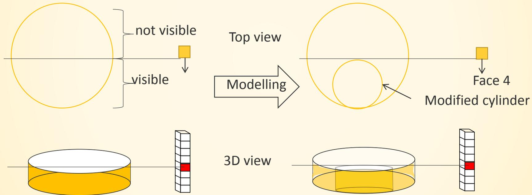
In this case, initial cylinder transformed into a modified cylinder in the visible zone
