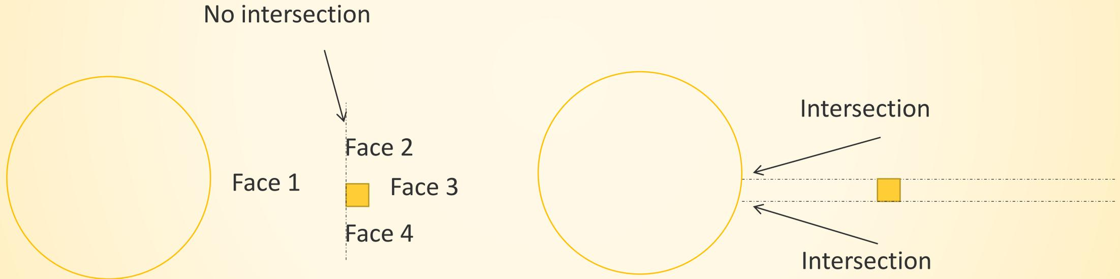
! The formula for cylinder is not valid if the receiving surface intersect the cylinder !
