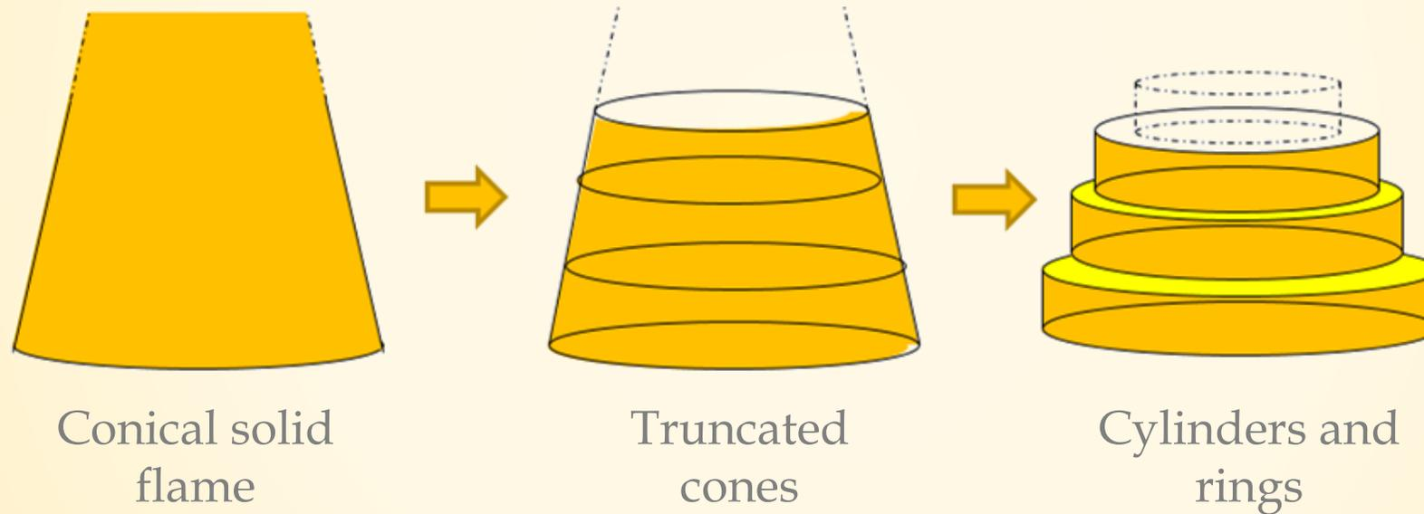
! By neglecting the contribution of rings, we underestimate the received flux and could even obtain a received flux equal to 0 above the fire !
