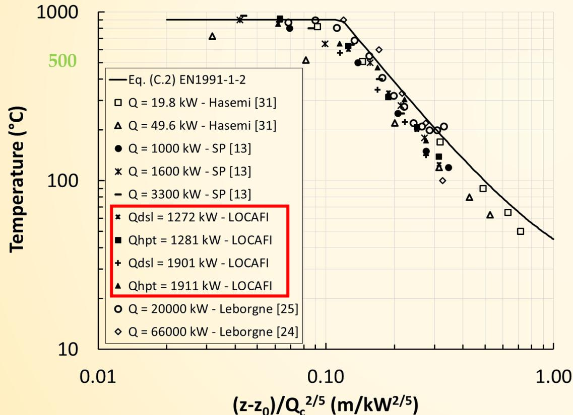
EN 1991-1-2 correlation provides a good assessment of temperatures both in the flame ( $\theta_g \geq 500^\circ\text{C}$ ) and the plume ( $\theta_g < 500^\circ\text{C}$ ).
