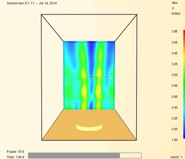
Example of flux variations due to an insufficient number of Radiation Angles
