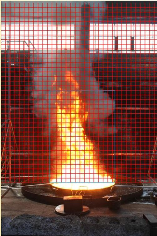
The mean flame length  $L$  is the distance above the fire source where the intermittency has declined to 0.5, where intermittency  $I(z)$  is defined as the fraction of time the flame lies above the fire source. This assessment was made using digital image analysis.
