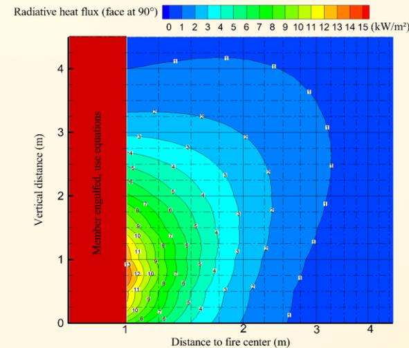
$D = 2\text{m}$ ,  $\text{RHR} = 500 \text{ kW/m}^2$ ,  $\theta = 0^\circ$  (left) or  $\theta = 90^\circ$  (right)
