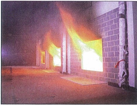
Fig. 19: Fire test on 7,0 × 17,9 m precast units supported by protected steelwork
