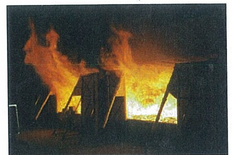
Fig. 18: Fire test on a 12,2 m x 12,2 m slim-floor system
