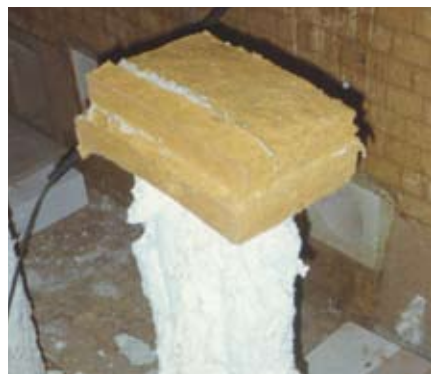
Brandwerende coating na verhitting
